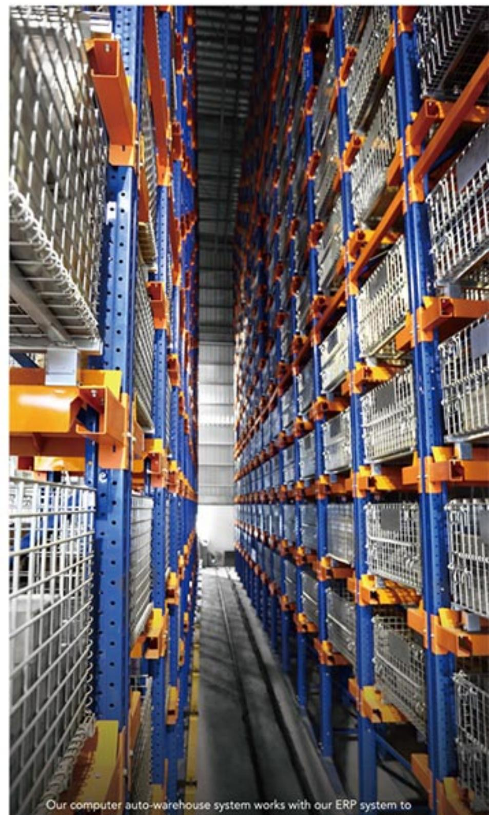
Our computer auto-warehouse system works with our ERP system to raise the efficiency in many different areas including cutting management costs, search times and inventory costs. Our system also improves factory floor efficiency and our procurement flexibility so that we are always in control.
